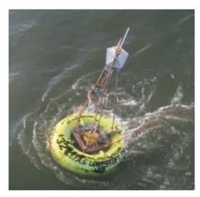
Smart buoy – providing real-time monitoring of the marine environment
